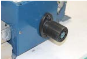
2) Open existing housing to remove fiber port
