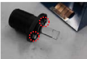
5) Do not tighten all the way. leave appx. 13/16" gap
