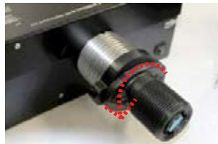
9) Twist fiber port counter clockwise until tight
