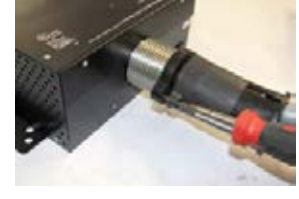
4) Screw and tighten with existing screws
