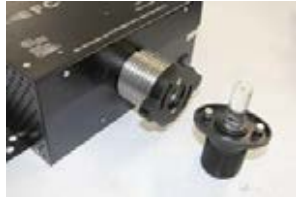
6) Reattach existing fiber port to new unit
