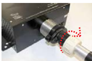
10) Screw on new fiber harness. (NOTE: It may be necessary to hold part to avoid twisting off)
